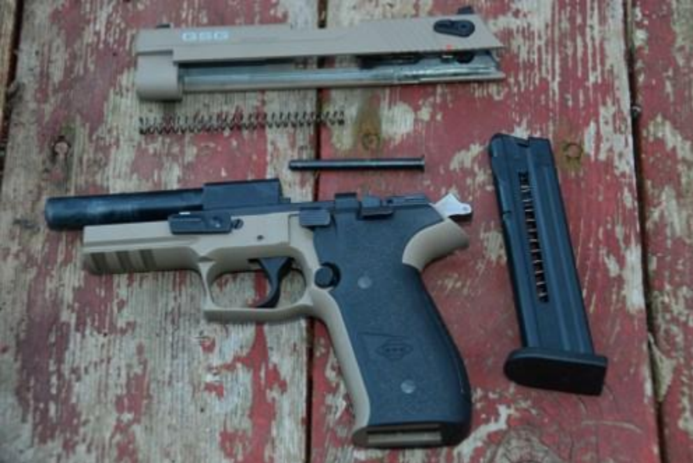
A disassemble Firefly, which is made easy with the teardown lever for cleaning and changing the spring.
