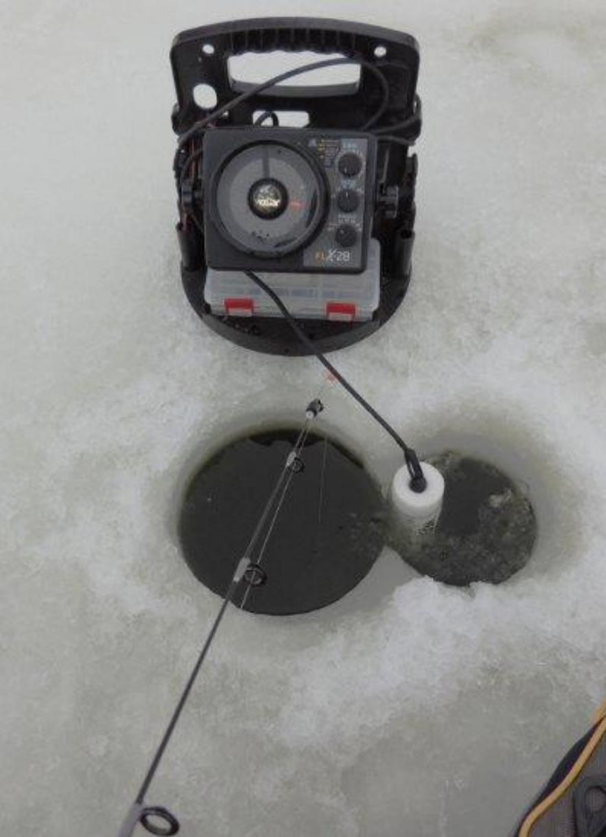
This is the two-hole system so that the flasher has its own protected transducer hole.
