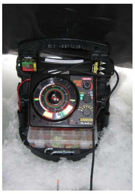
The zoom feature on the FL22HD flasher, shows fish suspended about 2 ½-feet off the bottom.
