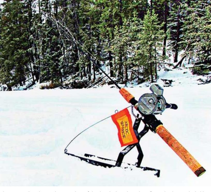
bar in a notch in the attachment. When a fish takes the line, the rod tips forward, releasing the holder bar, and setting off the flag. Then the angler simply walks up to the Arctic Warrior, takes the rod/reel combo out, closes the bale, and sets the hook. The fish can now be fought and played fighting and playing with a reliable drag and an appropriate action rod. No more cut fingers or dealing with a mess after a day of fishing.
