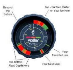
Many times it appears that a fish rises up from the bottom to reach your jig. In actuality, it is really coming in at the same depth as your hook but since the fish is further away from the center of the transducer signal, it looks as if the aggressive fish is moving from the bottom up.
