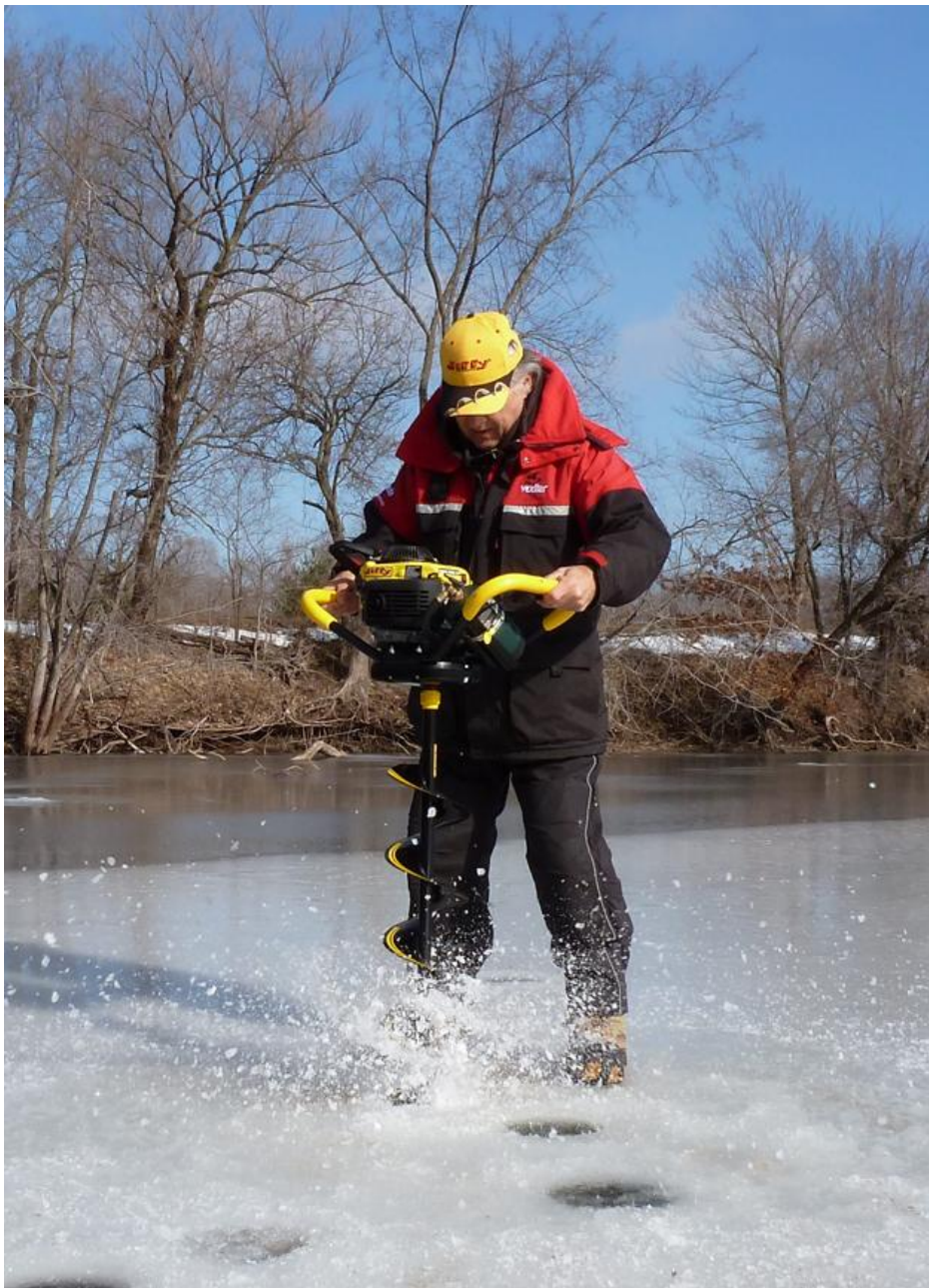
The Jiffy Pro4 and Pro4 Light drills that are fueled by propane are not only more economical and environmentally friendly, but are extremely easy to start.
